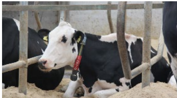
A Heatime™ HRLDn tag sits high on the left-hand side of the cow's neck where it detects subtle movements associated with rumination and heat activity.
