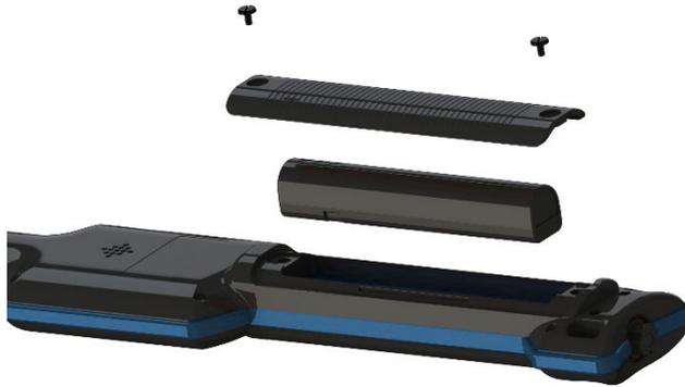
Remove the flat-head-screws by using the provided screwdriver. Lift the battery cover and take out the battery. After the new battery pack has been inserted, close the battery cover again and tighten the two flat-head-screws.
