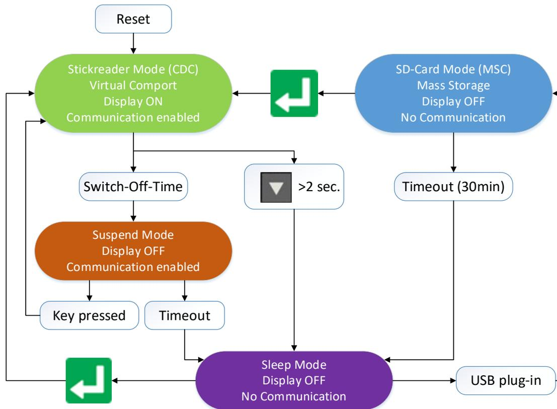
When the reader is switched on and it is connected via USB, it works in CDC mode. This means that a virtual comport is created on the computer and it can send commands to the device via a serial port connection. In this state, the mass storage mode is not activated and files cannot be copied to or from the AWR300.
