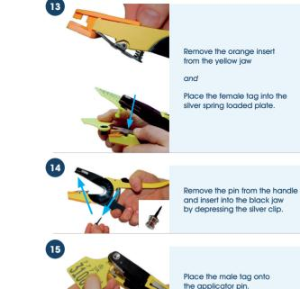
Place the male tag onto the applicator pin.
