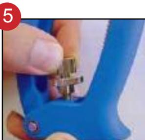
Turn dosing adjustment screw to set the required dosage. Retighten lock nut
