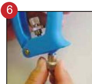
Handle spring pressure can be adjusted for comfort and tension
