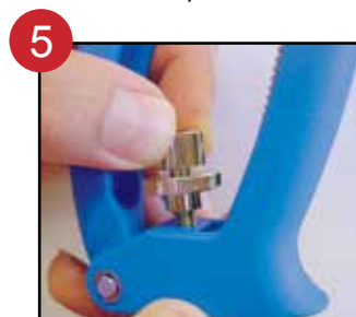
Turn dosing adjustment screw to set the required dosage. Retighten lock nut
