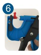
You have now completely grabbed the cutter. After the cutter is inserted into the piston you can release the handles
