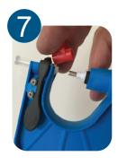
You can now easily remove the red connection piece while holding the two red tabs and pushing sideways
