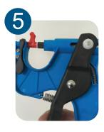
Carefully squeeze the plier handles until the large piston comes to a stop against the red connection piece
