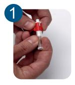
Take an assembled TSU (cutter + connection piece + collection tube)
