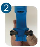
Squeeze the two spring loaded retainer clips together
