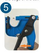
3. Remove the used cutter from the pliers by pushing the handles apart. This will loosen the needle and make it easy to remove. You cannot reuse the needle as it has no red plunger.
