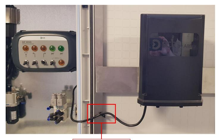
Correctly Secured Cable
