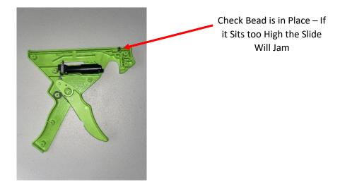
27. Place the slide side of the applicator on top of the plunger/trigger side ensuring that the screw holes line up. Screw the applicator back together using the 6x medium screws. It is helpful to start from the right hand side as this secures the bead in place.
