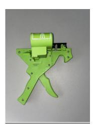
31. Run a strip of RapID or Superflex tags through the applicator to ensure that it functions correctly before heading to the yards.
