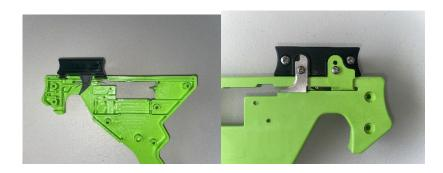
18. Ensure that the slide is able to move up and down it's track.
