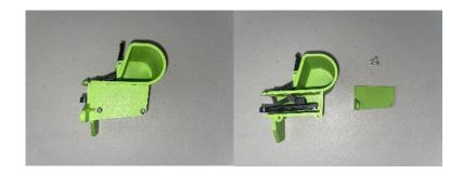
20. To slide the cam and pawl out of the housing, slide the cam to its outer most position. Then pinch the cam down to the pawl and wriggle it free. Be careful not to break any of the parts, sometimes it is helpful to stretch the green housing with your other hand as you wriggle.
