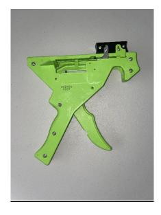
28. The next step is to place the barrel onto the rest of the applicator. Ensure that the tag slide is all the way forward. If the slide will not go all the way forward the bead will need to be pushed down into position. Then move the cam into the outward position and locate the diagonal cut out. Slide this cut out over the metal bar at the top of the plunger. Once in place, wiggle the barrel onto the applicator and align the remaining screw holes.
