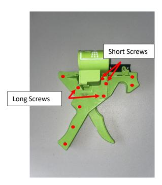
3. With the applicator lying flat on a table pull the top half away from the bottom half. Please note that the applicator is spring loaded so remove the halves slowly and gently to avoid losing any of the spring loaded parts.
