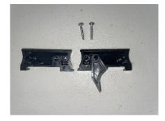
15. Remove the old tag loader arm, note it's orientation within the slide casing, the curve faces forwards.
