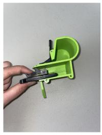
24. Check that the spring has stayed in place by sliding the cam in and out. The pawl should rise when the cam is out and fall when the cam is in. If the spring has shifted, remove the cam and pawl and redo the previous step.
