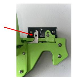
2. Remove the 10 screws from the side of the applicator, note which holes the 2x longer and 2x shorter screws are from. Once the screws 2x long and 2x short screws are removed, wriggle the barrel free and place to the side.
