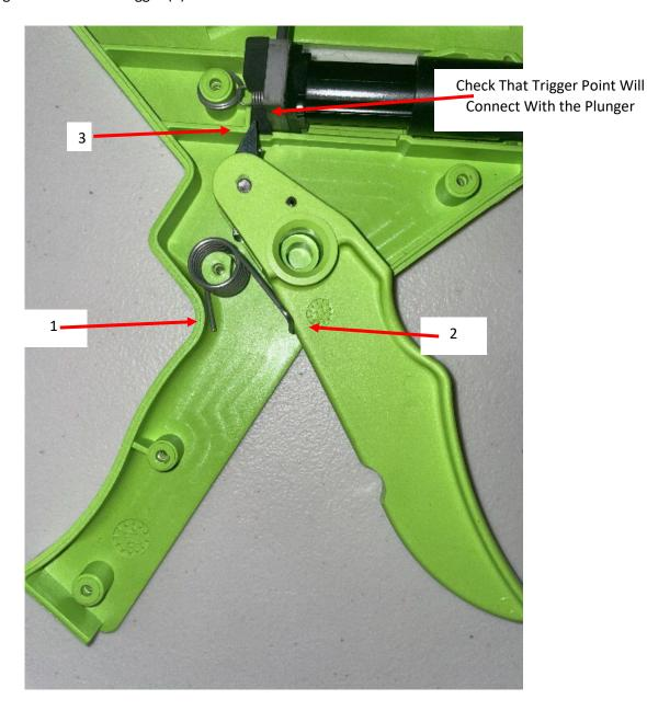
8. Ensure that the metal arm at the top of the applicator is positioned in the groove behind the plunger's metal plate (3).
