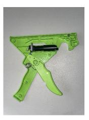
6. Lift off the trigger and discard the old spring. Check that the trigger is in good usable condition and that the metal arm at the top is still springing back and forth effectively. Place the trigger back into it's position.
