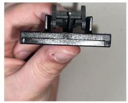
23. Pinch the pawl down to the cam while using your thumb to hold the base of the spring in place. Use your other hand to gently stretch the green housing whilst sliding the cam into place.
