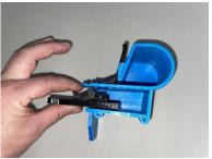
23. Check that the spring has stayed in place by sliding the cam in and out. The pawl should rise when the cam is out and fall when the cam is in. If the spring has shifted, remove the cam and pawl and redo the previous step.
