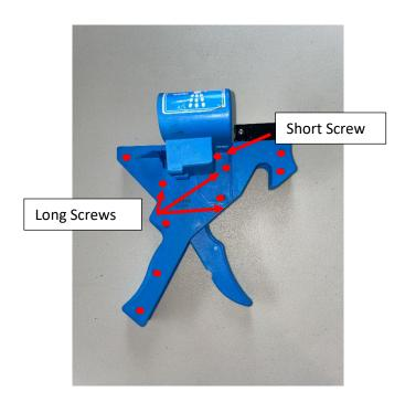
3. With the applicator lying flat on a table pull the top half away from the bottom half. Please note that the applicator is spring loaded so remove the halves slowly and gently to avoid losing any of the spring loaded parts.
