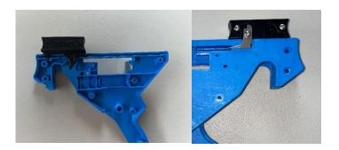
17. Ensure that the slide is able to move up and down it's track.
