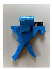
29. Run a strip of Flexi tags through the applicator to ensure that it functions correctly before heading to the yards.
