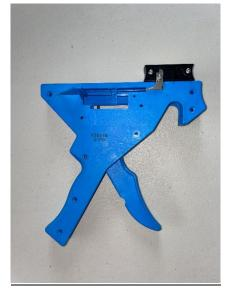
27. The next step is to place the barrel onto the rest of the applicator. Ensure that the tag slide is all the way forward. If the slide will not go all the way forward the bead will need to be pushed down into position. Then move the cam into the outward position and locate the diagonal cut out. Slide this cut out over the metal bar at the top of the plunger. Once in place, wiggle the barrel onto the applicator and align the remaining screw hole.
