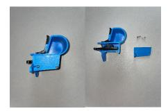
19. To slide the cam and pawl out of the housing, slide the cam to its outer most position. Then pinch the cam down to the pawl and wriggle it free. Be careful not to break any of the parts, sometimes it is helpful to stretch the blue housing with your other hand as you wriggle.
